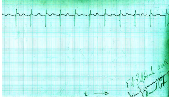
Figure 2. The first MCG, recorded in my MIT shielded room (Dec.1969), using Jim Zimmerman's SQUID. Although not obvious in this old record, the trace was as clear as the conventional ECG. It is signed by Edelsack, Zimmerman, and Cohen.
